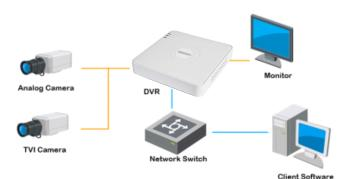
NOTE The S-TURBO series DVR only support cameras LB7TURBO, LB7TURBOW, LD7TURBOW, LE7TURBOW.
